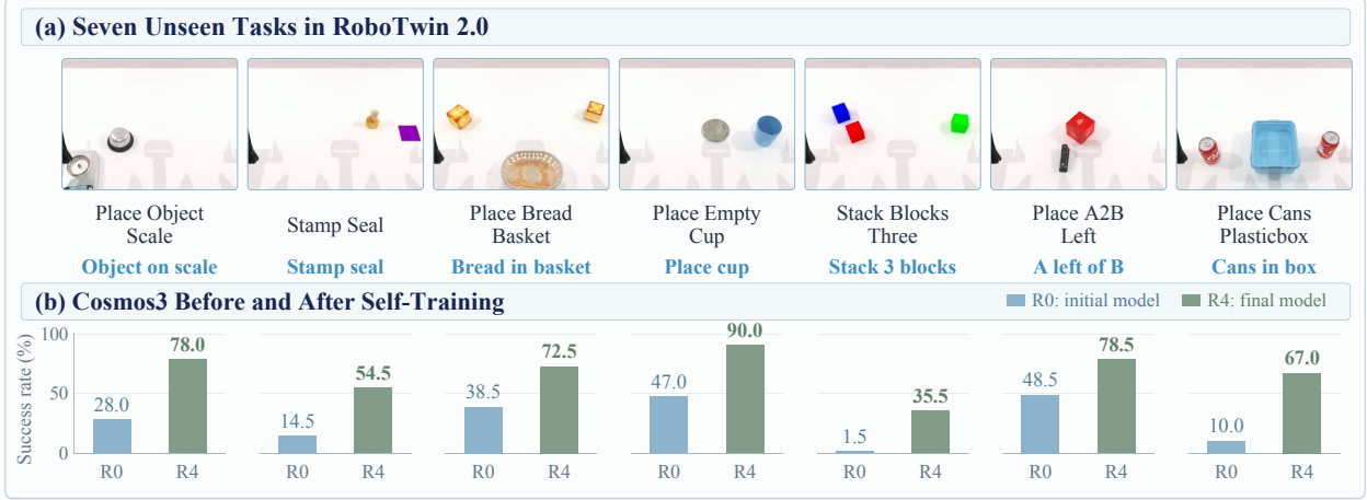
Figure 4: Unseen-task improvement in RoboTwin 2.0. (a) Example task scenes. (b) Cosmos3’s per-task success rates before self-training (Round 0) and after four rounds (Round 4).
