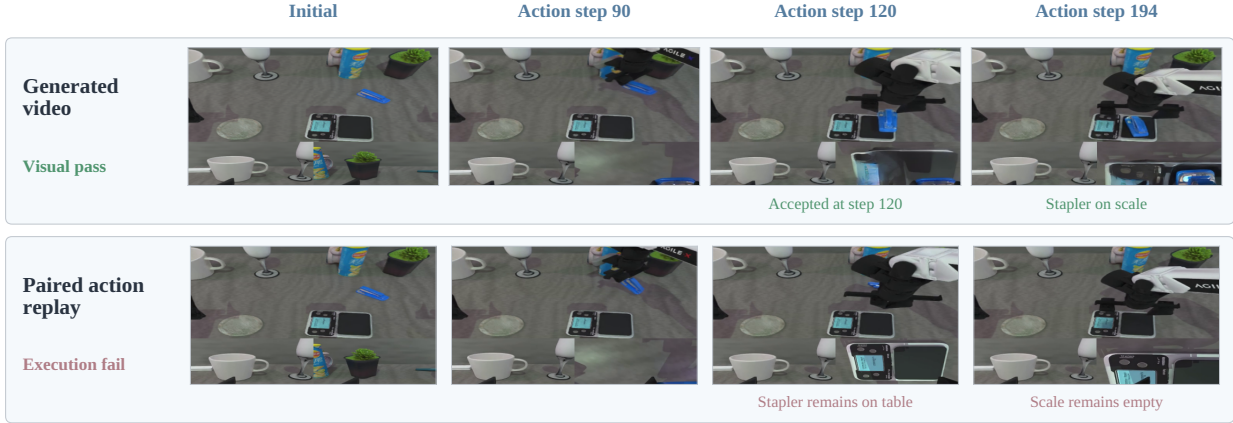
Figure 11: Generated completion and failed action execution. Top: the video generated by the 30,000-step Cosmos3 policy. Bottom: simulator execution of the same generated action sequence. Columns use the same action steps and show the main view above the two wrist views. The generated stapler reaches the scale; the replayed stapler remains on the table. The last column is the end of the 194-action replay. The visually accepted 120-action prefix has an IDM consistency error of 0.00632283, exceeding the fixed threshold of 0.00418487, and is therefore rejected by the IDM.
